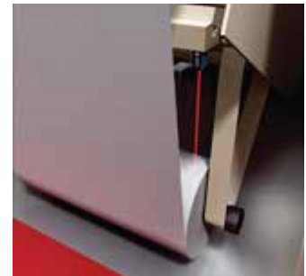
Measuring the diameter of the paper roll
