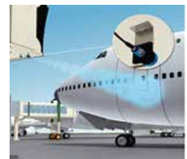
Docking the passenger boarding bridge to the aircraft
